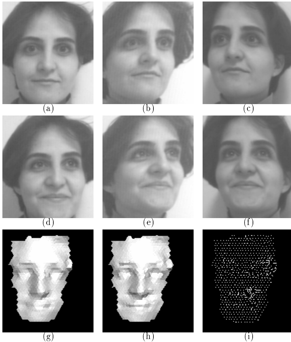
Figure 8: Application to motion tracking of deformable objects. (a,b,c) Triplets of face images taken simultaneously. (courtesy of INRIA). (d,e,f) Second triplet taken slightly later. Note that the head has moved and that the expression has changed. (g) Reconstructed surface for the first triplet. (h) Reconstructed surface for the second triplet, shown rotated and translated so that it matches the first one. (i) Flow field of the motion of the vertices of the first mesh to the rotated second one. Note that the field exhibits no overall structure and only local deformations, showing that the global motion has been correctly recovered.
