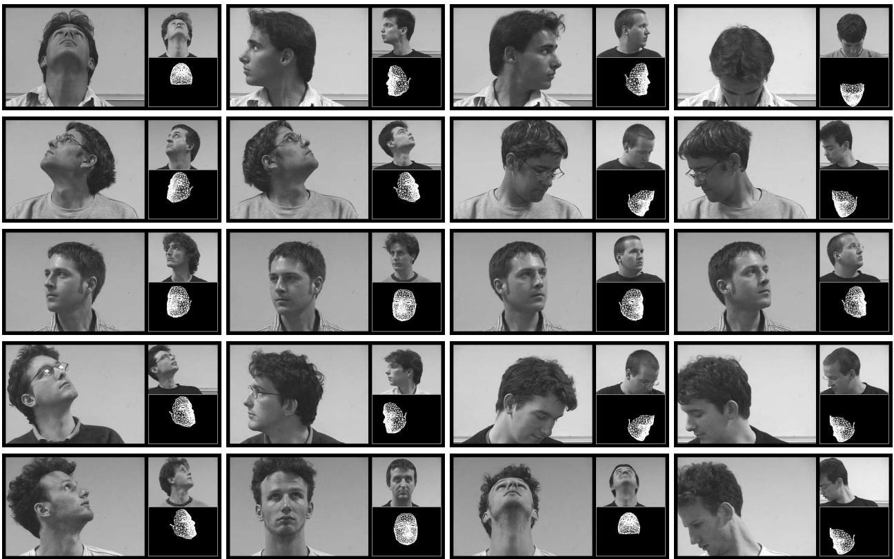
Figure 4. Results of pose estimation algorithm for the INRIA database where 930 images of 5 people filmed twice in 93 poses were used for testing and 1860 image of 10 people filmed twice, also in 93 poses, are used for training. On the left of each image is the query image. On the up-right is the selected person from a database which have the most similar pose as the one of query image. On the bottom-right the recovered 3D mesh model indicating the global face positions is depicted.
