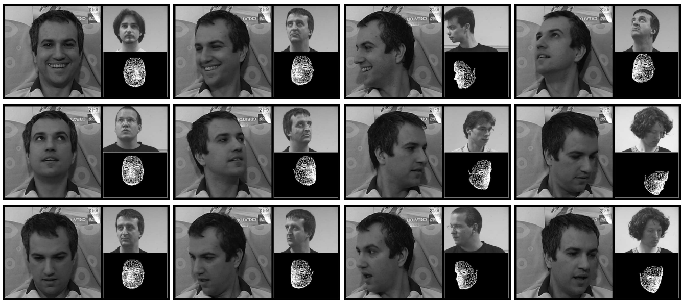
Figure 6. Pose estimation against a cluttered background, arbitrary lighting and facial expressions. Each image includes, on the left a frame of a video sequence used as a query image and, on the right, the database image that matches it best and a 3D wireframe mask projected in the recovered pose.
