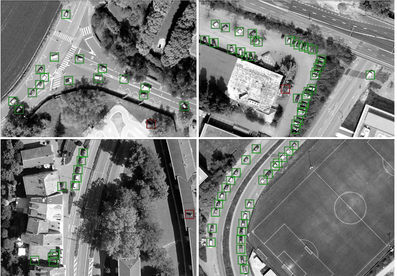
Fig. 19: Some examples from our car test set. True positive rate is 85%. Correct detections are shown in green whereas false alarms are shown in red. There are 198,000 tests per image.
