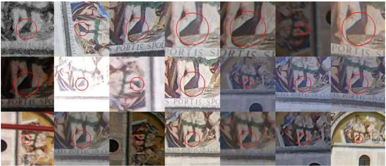
Fig. 2. Some of the keypoints from the same 3-D point for the Venice dataset in Figure 16 are shown as an example. The red circle shows the keypoint (DoG) position and its scale. The track was extracted by consecutive SIFT L_2 matching, which makes it possible to include keypoint pairs (conjunctive closures) that are quite different into the training and evaluation set.
