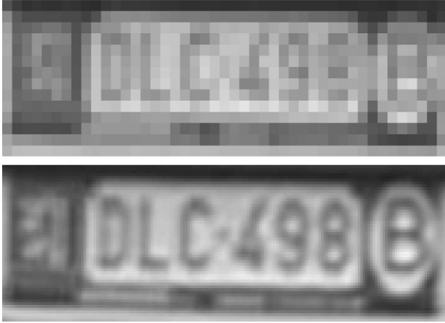
Fig. 11. Real data. Detail view of the licence plate in the original low-resolution image (top) and the corresponding super-resolution reconstruction (bottom).
