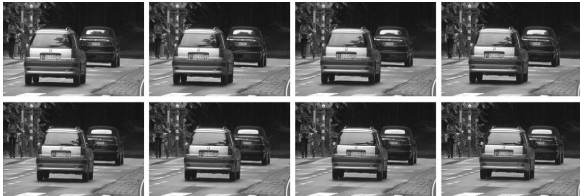
Fig. 9. Real data. Static camera with moving cars. Some of the 24 low-resolution input images. The purpose is to enhance the licence plate of the car in the front.
