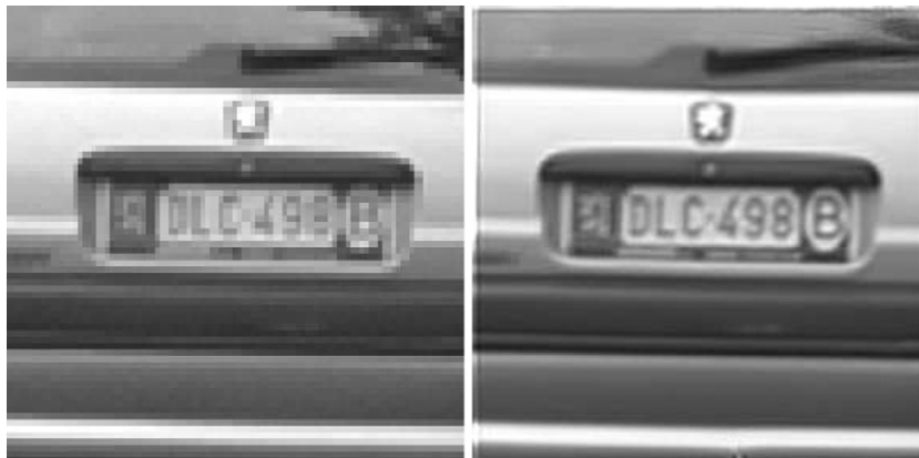
Fig. 10. Real data. Detail view of the rear of the car in the original low-resolution image (left) and the corresponding super-resolution reconstruction (right).
