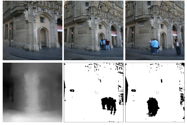
Figure 4. Top: 3 from the 5 input images. The first image was chosen as the reference view. Bottom: the final depth estimate (left) and the visibility estimates w.r.t. the 2 d and 3 d input image. The visibility maps are from the viewpoint of the reference camera.
